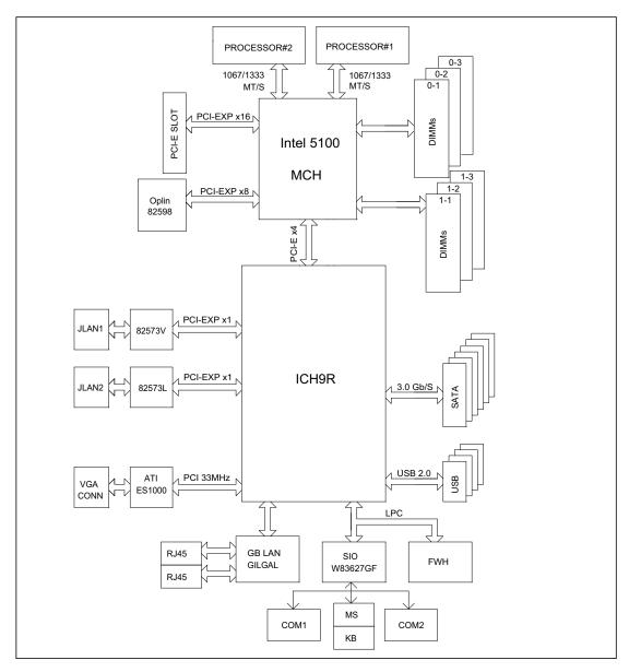
Figure 1-1. Intel 5100 Chipset: System Block Diagram
